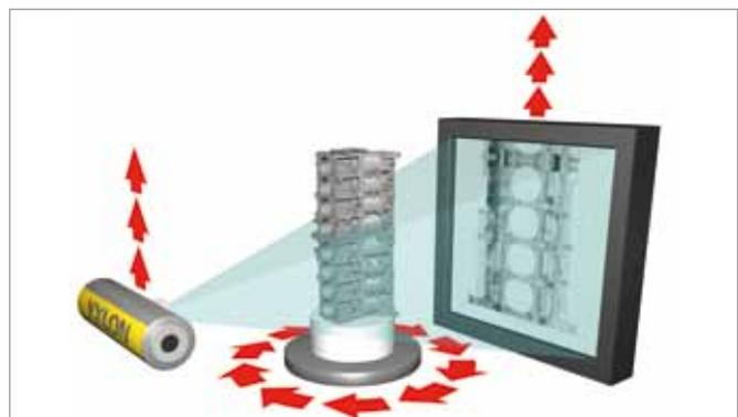
Principle of HeliExtend: With stepwise vertical manipulation of the X-ray tube and the flat-panel detector all information for precise 3D volumes of your parts are obtained. This method is also good for a vertical scan extension.
