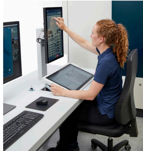
In the FF85 CT, software and hardware work hand in hand to make system operation as easy as possible. The clean layout of the operator desk with tiltable touchscreens allows users to stay focused on the inspection task. The height of the desk can be adjusted, facilitating operation from a sitting or standing position. Healthmonitor and push messages keep the user informed about system status and inspection progress at all times.
