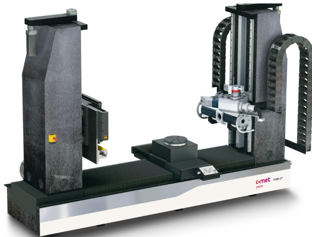
Small parts, large parts, dense materials – with its possible combination of two X-ray tubes, a spacious flat-panel detector and/or the CTScan 3 line detector, the FF85 CT is up for almost everything. Seamless switches between 2D radiography, 3D cone-beam, and fan-beam CT provide outstanding flexibility and allow for individual inspection processes.
