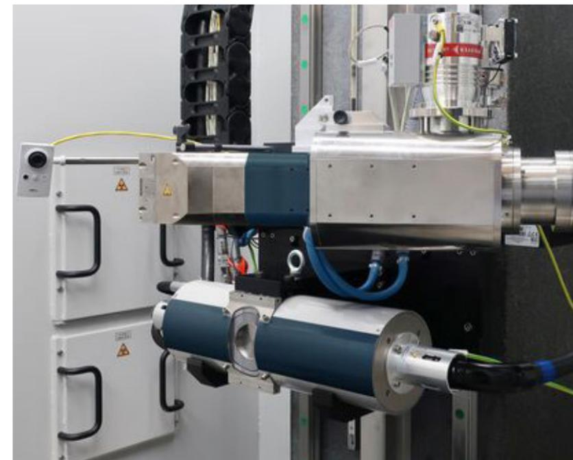
You can switch between the different tubes in one CT sequence.
